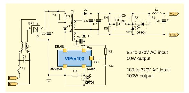
Off-Line Flyback SMPS with secondary regulation
